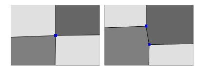
The polygons have to be transformed in such a way there is no common node with more than 3 polygons attached to it. As a further constraint, for a Closed-C or Eight "repair", the two polygons of the same region must be isolated from each other. The following diagrams show the situation "before" (left) and "after" (after) for an Eight, but the principle is the same for any situation.
