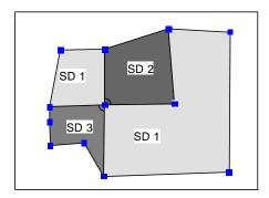
This example reveals that 4 polygons belonging to 3 regions meet at one node. It is a special case that should not happen because SD1 is an Eight region. We sill see how to "repair" an Eight and, generally speaking, any "problem" node
